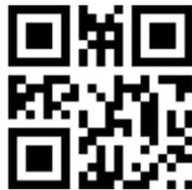
RTS/CTS Option 2: When Option 2 is selected, RTS is always high or low (user-programmed logic level). However, the scanner waits for CTS to be asserted before transmitting data. If CTS is not asserted within Host Serial Response Time-out, the scanner issues an error indication and discards the data
