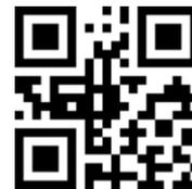
RTS/CTS Option 3: When Option 3 is selected, the scanner asserts RTS prior to any data transmission, regardless of the state of CTS. The scanner waits up to Host Serial Response Time-out for CTS to be asserted. If CTS is not asserted during this time, the scanner issues an error indication and discards the data. The scanner de-asserts RTS when transmission is complete.
